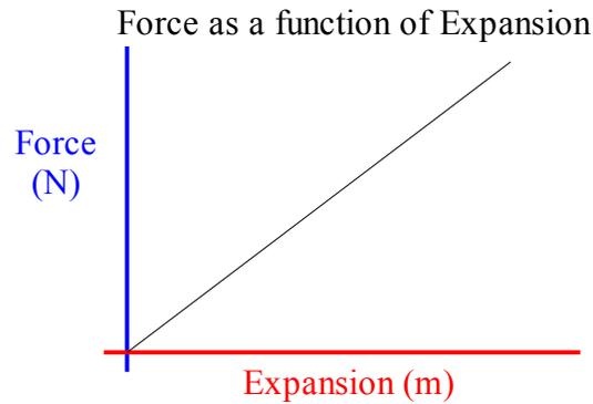
The slope of this line (rise over run) would be Force over Expansion... the slope is equal to the spring constant.
