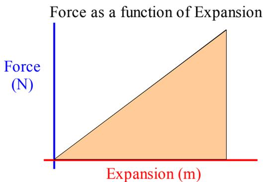
$$\begin{aligned} \text{Area} &= \frac{1}{2} bh \\ &= \frac{1}{2} F x \\ &= \frac{1}{2} (kx) x \\ \text{Area} &= \frac{1}{2} kx^2 = W \end{aligned}$$
