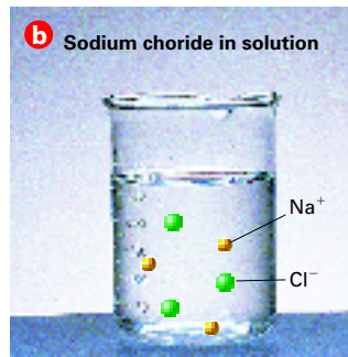
b Three moles of sodium chloride dissolved in water produce 6 mol of particles because each formula unit of NaCl dissociates into two ions.
