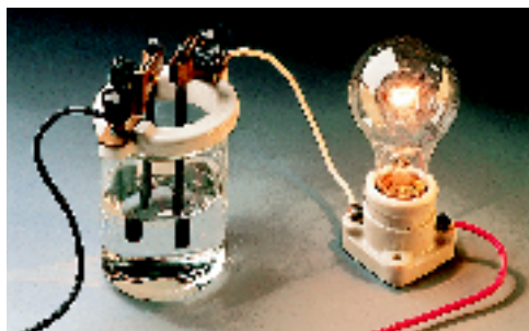
FIGURE 20 Ions in Solution A solution of sodium chloride conducts electricity across the gap between the two black rods of a conductivity tester. As a result, the bulb lights up.
