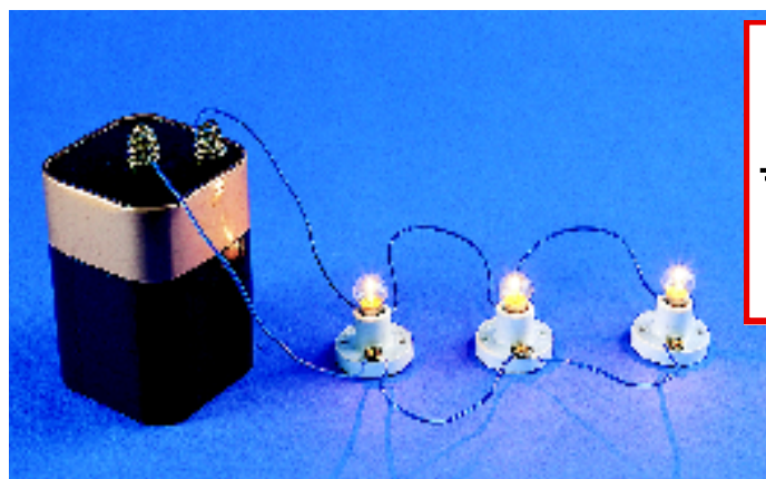
FIGURE 19 A Parallel Circuit A parallel circuit provides several paths for the flow of electrons. Predicting What will happen in a parallel circuit if one bulb burns out?
